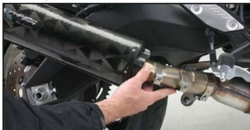
6. Slide rubber lined muffler clamp over muffler assembly and loosely attach to rear lower passenger foot mount using supplied 8x16mm bolt.
