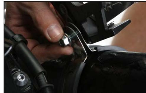
7. Check for clearance and alignment, then tighten all the bolts in this order: X-ring bolts, muffler mount, and finally barrel clamp.
