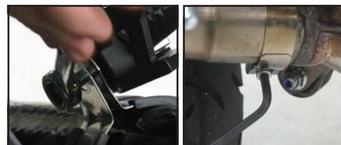
8. Remove OEM heatshield and install on TBR system.
