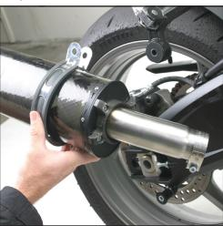
Loosely attach muffler to bike using the OEM bolt and nut and install muffler clamp to inside of passenger footpeg.
