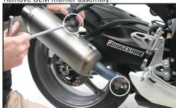
4. Attach muffler to TBR slip system using the supplied X-ring, 6x20mm socket head cap screws and lock washers that are provided, leave loose for now. Slide rubber lined muffler clamp and barrel clamp on and install to bike.
