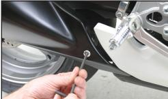
3. Remove OEM muffler assembly.
