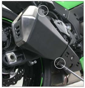
3. Attach TBR muffler to slip-on tube using the 4 6x20mm S.H.C.S. and lock washers provided. Leave loose for now. Slide rubber lined muffler clamp over muffler.
