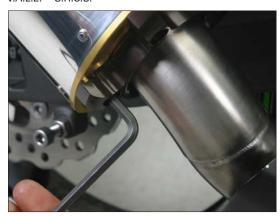
7. Tighten barrel clamp.
