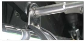
Check alignment and tighten muffler and the 4 6x20mm V.A.L.E.™ S.H.C.S.
