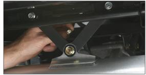
10. Loosely attach the two part X-ring using supplied bolts and washers and lock tight.
