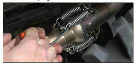
Remove muffler mounting bolts, this may require tilting the bed to access the nuts on the back side frame rail.
