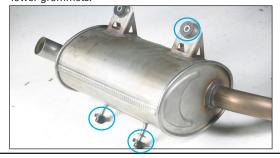
Make sure the ATV is completely cool before starting 7. Attach the three grommets to the TBR muffler.
