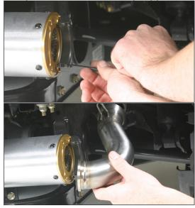
12. Make adjustments and securely tighten X-Ring bolts.
