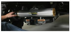
Attach supplied muffler hanger bracket using the 8x20mm bolts and nuts that were provided for upper mounts. Use the OEM bolt and nut with washer on lower mount. Tighten hardware.
