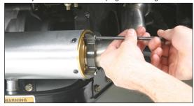
Attach OEM springs joining the OEM header to TBR muffler assembly.
