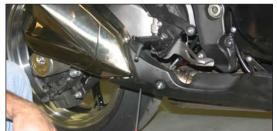
6. Remove right side exhaust muffler.
