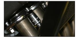
4. Remove OEM muffler assembly.
