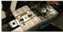
6. Loosen muffler joint clamp.
