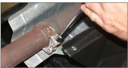
Remove muffler assembly.
