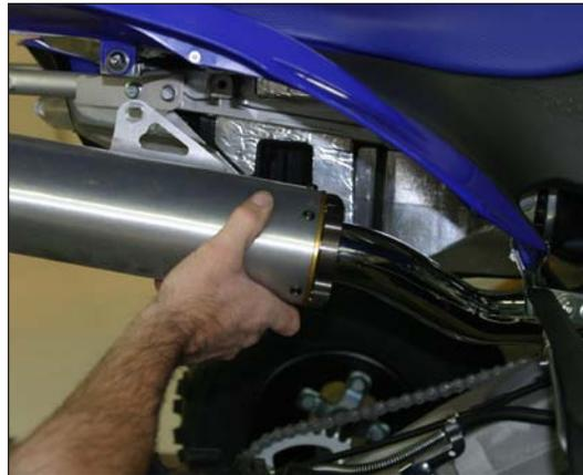
6. Before you run the atv, clean off all fingerprints and dirt, as any oily residue will etch the metal and become somewhat permanent when the system gets hot. Run the atv and enjoy. It is normal for some white smoke to appear the first time you start the bike. This is packing/manufacturing oil from inside the pipe burning off. After 30-60 minutes of use, recheck all fasteners for tightness.
