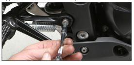
10. Attach the supplied mounting bracket to the inside of frame and secure in place with the supplied 8mm flange nut. Bracket should be installed as shown in picture.
