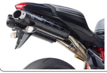
Align mufflers and tighten the 6x14mm V.A.L.E.™ hardware when the slip-on tube clearance and the muffler alignment is correct. It may be easier to tighten one bolt first, then remove the slip-on tube assembly to tighten all of the rest of the hardware.
