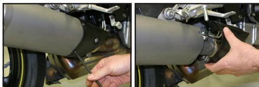
4. Remove cables from muffler and cable clamp from right side rearmount assembly.
