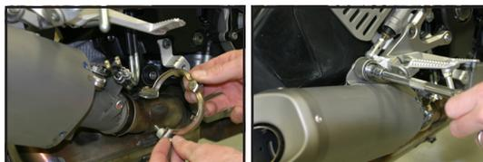
6. Remove muffler assembly. Also be sure to remove the OEM retaining ring and gasket from the stock slip tube.
