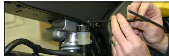
8. Remove the noise reduction valve servo bracket from the frame.
