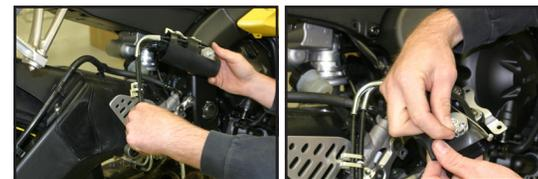
10. Remount the servo without the cables. This step is necessary in order to keep an error code from being displayed on the LCD screen.
