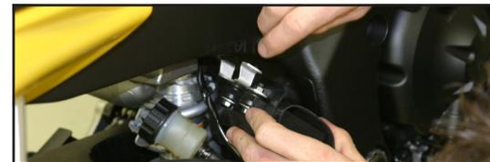
11. Reinstall the brake reservoir.
