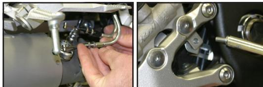
5. Remove muffler joint clamp and muffler mounting bolt.
