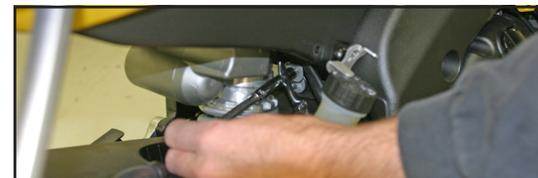
9. Remove servo by pulling out from the right side of the motorcycle and disconnect the cables. Disregard cables.
