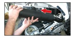
Use the 4 (four) 6 x 14mm socket head cap screws and split lock washers to loosely attach the X-Lite™ ring to muffler inlet.
