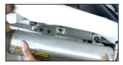
Securely tighten the 4 (four) 6mm x 16mm hex head bolts of the V.A.L.E. assembly.
