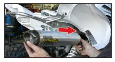
Attach muffler canister to frame using OEM bolts. Tighten both bolts securely.
