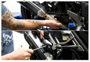
12. Tighten barrel clamp.
