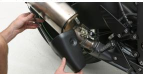
Remove exhaust valve cables from servo under seat. Use a wrench to hold server wheel in place or internal gears may break.
