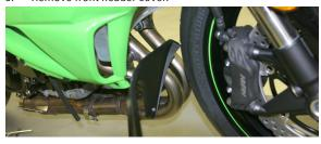
Remove header pipes.
