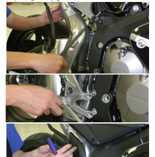
Replace reflectors and rear fender assembly, reconnect wiring and replace rear cowling, passenger & driver seats.
