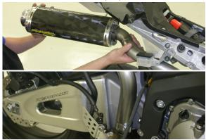
23. Slip upper & lower halves of muffler clamp onto muffler canister and attach to "L" brackets using supplied 8mm nuts and 8mm bolts.
