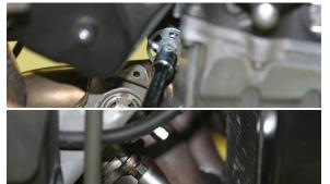
17. Install TBR header assembly using the OEM exhaust gasket between header and engine. Attach using the OEM nuts.
