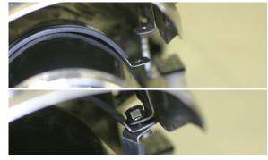
24. Making sure that the muffler canister is aligned correctly, securely tighten the 8mm bolts connecting the muffler clamp halves to the "L" brackets.
