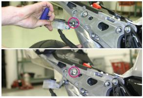
11. Remove right side driver's foot peg bolts and carefully remove the exhaust tube heat shield.
