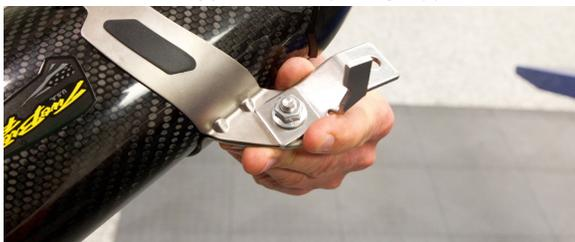
13. Apply a thin layer of anti-seize to slip tube outlet and attach to S1R muffler with supplied springs.
