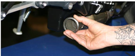
11. Note direction of TBR muffler clamp and install to 60mm at points indicated in picture.
