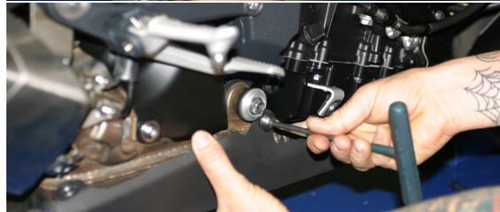
4. Unplug servo box located in front of the shock. Do not turn ignition on while servo is unplugged.
