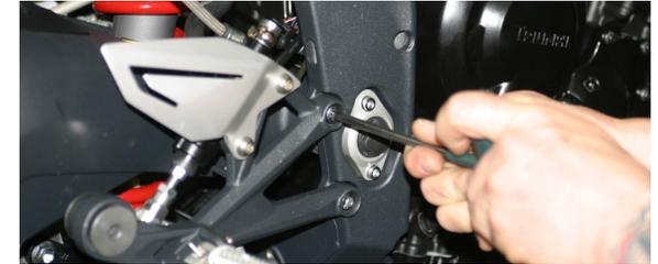
7. Remove OEM muffler mounting hardware.
