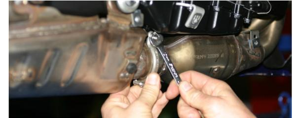
8. Remove OEM muffler assembly and servo box.
