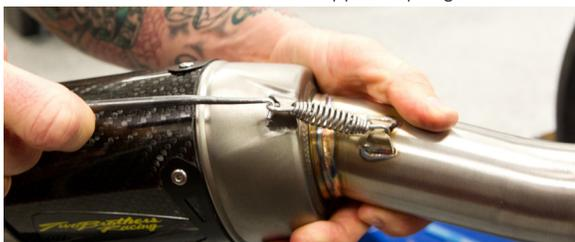
14. Slide TBR slip tube and muffler assembly onto header using supplied barrel clamp. Leave loose for now.
