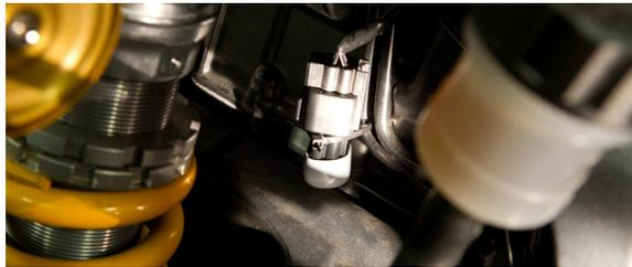
18. Check for clearance and alignment, then tighten all the bolts in this order: muffler mount, clamp bolt, and finally barrel clamp.
