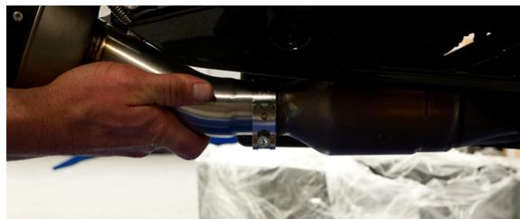
15. Attach muffler clamp to foot peg mount using stock bolt and washer with supplied 8mm flange nut.
