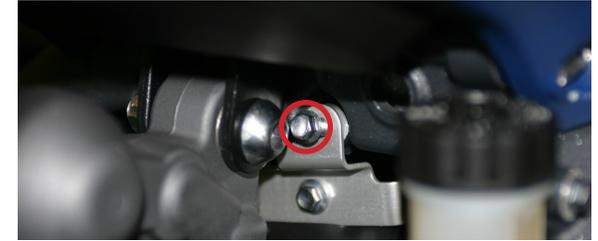
6. Temporarily remove right side rear set mounting hardware to ease removal of servo box.
