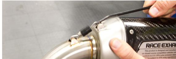
11. Slide muffler/slip-tube assembly into position on header pipe.
