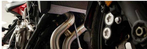
8. Attach supplied muffler mounting bracket using two OEM bolts and two 6mm flange nuts (provided).
