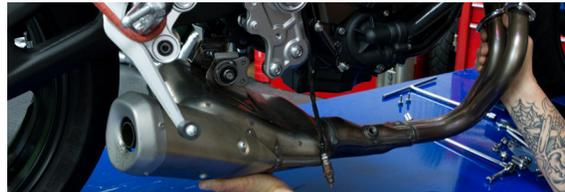
7. Attach the TBR header assembly using OEM hardware and gaskets. Leave loose for now.
