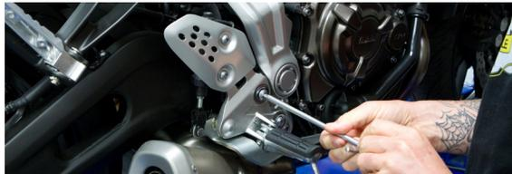
5. Remove muffler mounting bolts.
