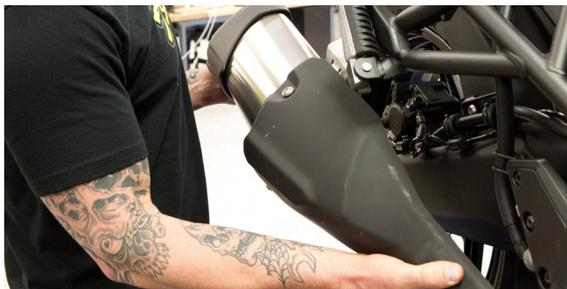
3. Install Two Brothers Racing Slip-on Exhaust System: Attach the mid-pipe to the muffler using the 2 hook springs provided. Apply a thin layer of anti-seize to muffler inlet.
