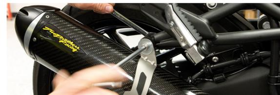
5. Align muffler and tighten clamp.
