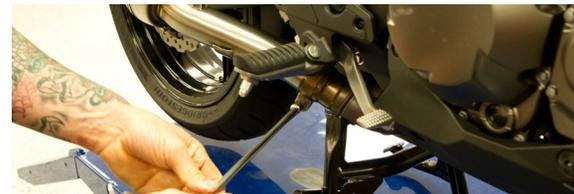
6. Re-check all hardware and fitment. Make sure muffler is aligned when the bike is on the center stand. Also keep even clearance between the muffler and luggage bag.
