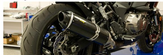
7. Before you run the bike, clean off all fingerprints and dirt, as any oily residue will etch the metal and become somewhat permanent when the system gets hot. Run the bike and enjoy. It is normal for some white smoke to appear the first time you start the bike. This is packing/manufacturing oil from inside the pipe burning off. Check for gaps or leaks. If you find a leak, a little high temperature silicon sealant should fix it. After 50 to 100 miles, recheck all fasteners for tightness.
