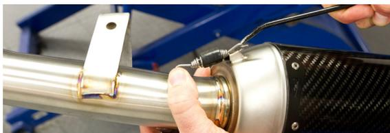
4. Slide provided rubber lined muffler clamp over muffler body.
