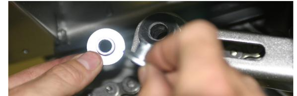
7. Attach supplied muffler mounting bracket to the two rubber mounting supports on right side. Use supplied nut and bolt and previous removed nut and bolt.
