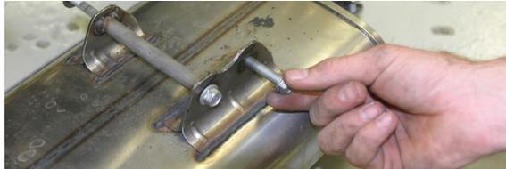
6. Remove the rubber grommet and inserts from the frame where the stock muffler mounted on the left side.
