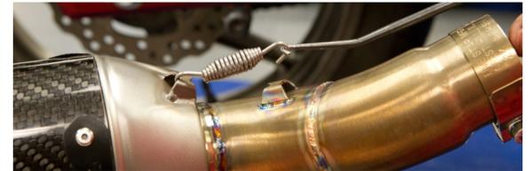
9. Slide the (rubber-lined) muffler clamp over the muffler canister and install on bike using supplied barrel clamp.
