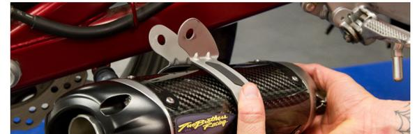
10. Make all adjustments of slip-on tube rotation and muffler rotation to make sure there is clearance between swingarm/tire and brake pedal when applied.
