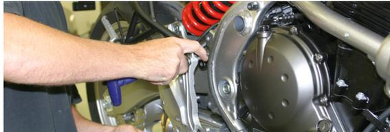
4. Loosen the muffler clamp attaching the OEM muffler to the head pipe.
