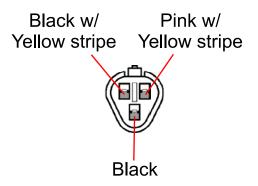
6. Insert the three male terminals into the Larger 3p white plug through the back until they click into place. The diagram below shows the lead orders with the front of the plug facing you:
