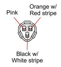
**7.** After installing the plug adapters, plug in both the male and female 3-pole SH harness connectors. Make sure the connectors are fully seated.
