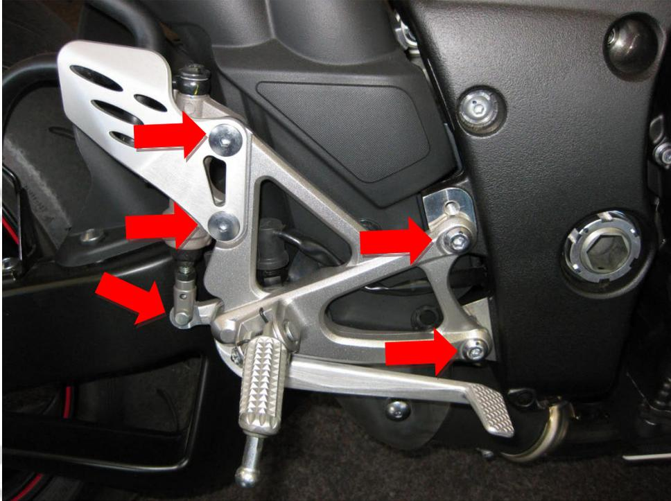
Connect the brake cylinder with the R&G brake cylinder adapter, find the right position for the Rearsets and connect them with the frame.
