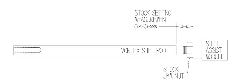
To ensure the correct operation of the shift assist system please install the Vortex Shift Rod (RS188C1 Or RS188C2) as shown in the diagram. Take great care to ensure that you have the system adjuted as shown to start. Once this is set please use the heim joints on both ends of the shift rod / shift assist assembly to adjut the length for pedal position.
