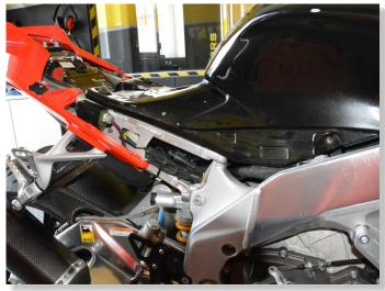
LIFT UP OR REMOVE THE FUEL TANK.
