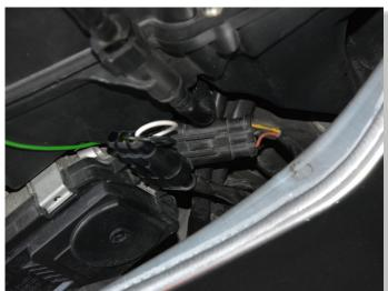
CONNECT QSH CONNECTORS IN-LINE WITH THE IGNITION COIL CONNECTORS ON AIRBOX.
