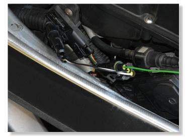
CONNECT QSH CONNECTORS IN-LINE WITH THE IGNITION COIL CONNECTORS ON RIGHT SIDE.
