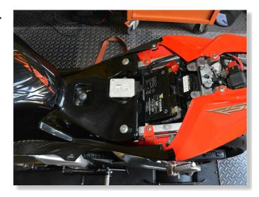
REMOVE THE FRAME COVERS BELOW FUEL TANK.
