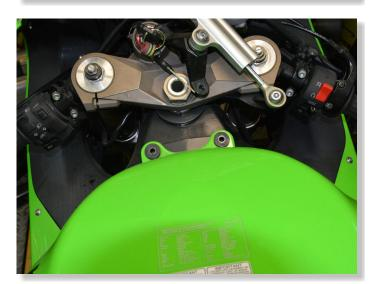
REMOVE THE STEERING DAMPER HOLDER.
