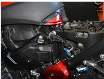
LIFT UP OR REMOVE THE FUEL TANK.
