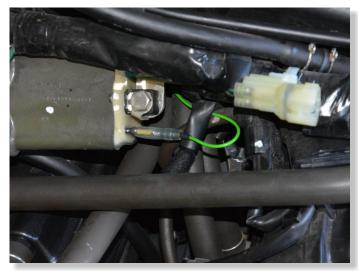
SPLICE THE QSH WHITE WIRE TO THE YELLOW/BLUE WIRE OF THE COIL BY USING THE SUPPLIED RED WIRE TAP CONNECTOR.
