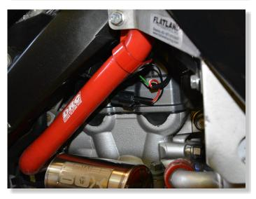
PLUG THE QSH CONNECTOR PAIR WHICH IS MARKED WITH RED SQUARE IN-LINE WITH THE IGNITION COIL CONNECTOR. (BLACK, 2-POLE CONNECTOR BELOW FUEL TANK)
