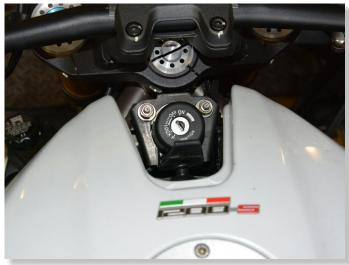
LIFT UP OR REMOVE THE FUEL TANK.
