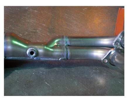
2. Stabilize the system and make cut along weld edge.
