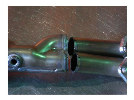
3. Grind cut area smooth around the outside. You also may need to do some clean up on the inside of the tubes.
