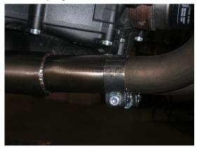
7. Attach mounting tab to the outside of the previously relocated stock mounting point (see photos below). Use the stock bolt and supplied M8 flange nut.
