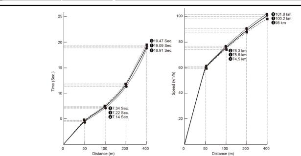
NOTE • ENDURANCE Cylinder (61mm)+ENDURANCE Camshaft (240°)+ENDURANCE Hurricane multi air filter (High-density sponge x1)+other parts are Honda stander parts
