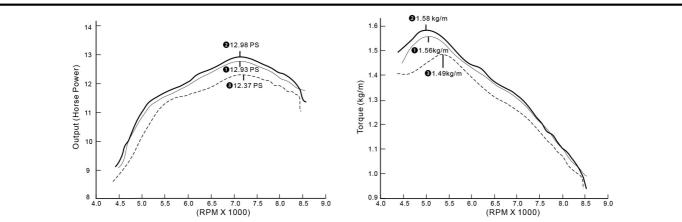
NOTE • ENDURANCE Cylinder (61mm)+ENDURANCE Camshaft (240°)+ENDURANCE Hurricane multi air filter (High-density sponge x1)+other parts are Honda stander parts. (Test with 3RD gear positon)
