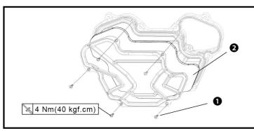
• To replace filter cartridge, remove 1 screws (Accessory 5) and 2 replace sponge (two sponges with different densities are available). After replace sponge, make sure you tie up all necessary screws(Accessory 5).
