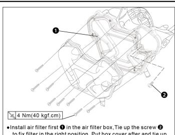
to fix filter in the right position. Put box cover after and tie up all necessary screws (Accessory 4).
