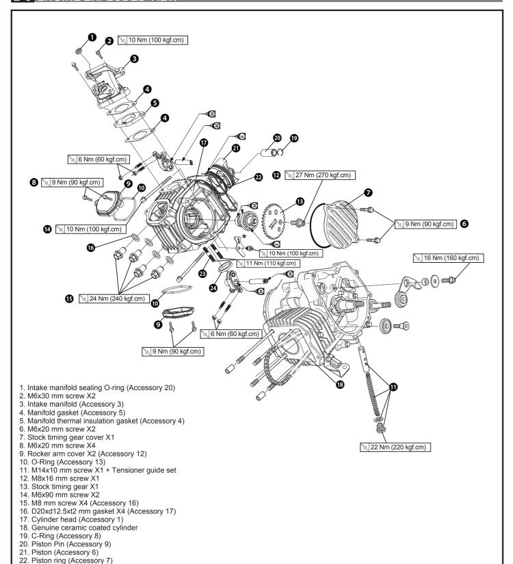
NOTE \* Symbol on camshaft plate stopper must be facing the outside.
