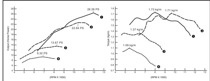
NOTE OKOSO MSX 4V Cylinder head (M)+KOSO MSX 4V Ceramic coated cylinder (61mm)+KOSO MSX 4V Camshaft+ECU+KOSO MSX Throttle body (34 mm)+KOSO Injector (160 c.c.)+KOSO Intake+After Market Exhaust+Factory standard setting.
