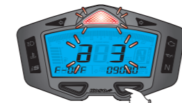
3.RPM red shift light value setting and flashing ON/OFF
