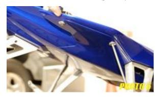
**6.** Remove the four plastic #2 phillips fasteners (**photo 6**). Remove the body panel.
