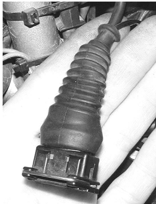
7. Connect and secure the RPM/Timing Sensor connector with zip-tie.
