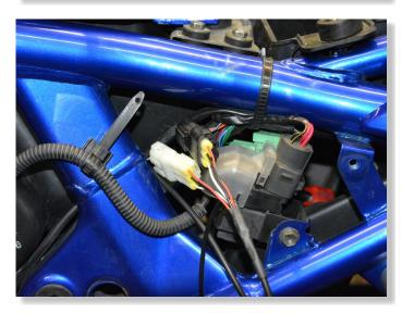
PLUG GPX CONNECTORS IN-LINE WITH THE SPEED SENSOR CONNECTORS. (BLACK, 3-POLE CONNECTORS AT LEFT SIDE NEAR MAIN RELAY)
