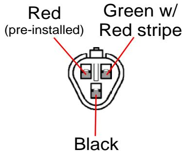
7. Insert the two male terminals (which you released in step 5) into the **Larger 3p** plug through the back until they click into place. The diagram below shows the lead orders with the front of the plug facing you:
