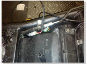
CONNECT ATRE RED WIRE TO ORANGE/GREEN WIRE OF DIAGNOSTIC SYSTEM CONNECTOR.
