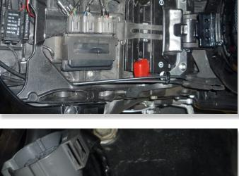
RELEASE AND REMOVE THE MIDDLE TWO PINS FROM FEMALE CONNECTOR. (GRAY, 10-POLE CONNECTOR UNDER FUEL TANK AT THE LEFT SIDE) (BLACK/YELLOW AND WHITE/YELLOW WIRES)
