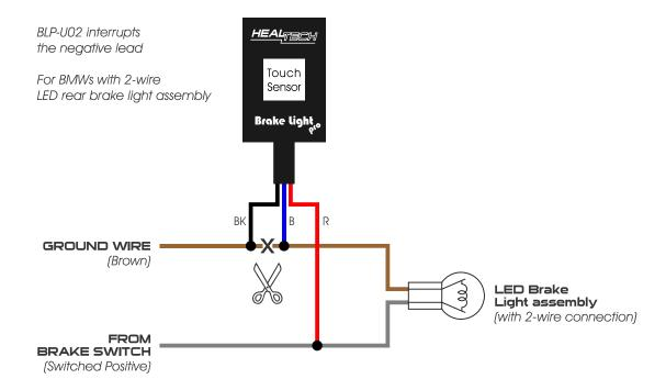
2. Find and **disconnect** the rear brake light assembly connector then proceed as shown on this photo:
