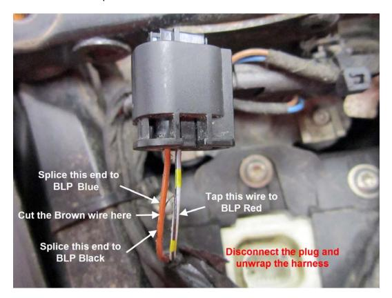
To make the 3 splices, use the supplied red quick connectors. Do NOT strip the wires when using the red connectors.
