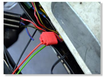
CONNECT THE BLP GREEN WIRE TO BLUE/RED WIRE END, WHICH GOES TO THE REAR LIGHT CONNECTOR.
