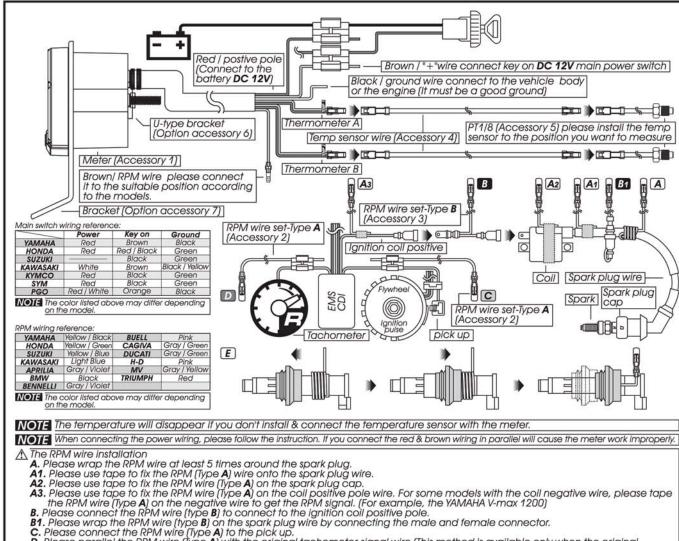
C. Please connect the RPM wire (Type A) to the pick up.
