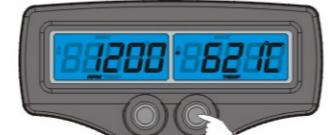
● Press Adjust button once to switch screen from water TEMP/EGTB to water TEMP/EGTA.
