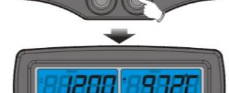
● Press Adjust button once to switch screen from RPM/EGTB to Water TEMP/EGTA.
