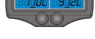
● Press Adjust button once to switch screen from water TEMP/EGTB to water TEMP/RPM.
