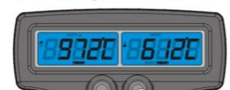
● Press Adjust button once to switch screen from RPM/EGTA to RPM/EGTB.
