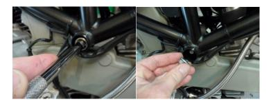
3. Slide the right hand slider (99-FS-750-8209-R) and spacer (428-9111) over the supplied engine stud as shown below and install engine stud through frame. Note: 428-9111 right hand spacer will only fit into frame on the right hand side.
