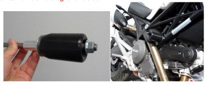
4. Install left spacer (428-9110) and left hand slider (99-FS-750-8209-L) with provided nut (99-HN-LN12125). Torque nut down to the OEM torque specifications.
