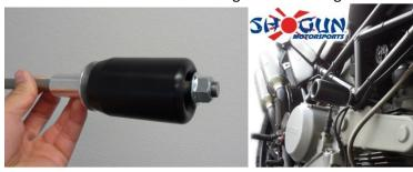
4. Install spacer (428-9103) and left hand slider (99-FS-750-8209-L) with provided nut (99-HN-LN12125). Torque nut down to the OEM torque specifications.
