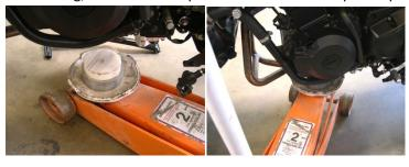
2. Remove the rubber caps to expose the main engine stud bolt and nut. Remove the nut and OEM Bolt.
