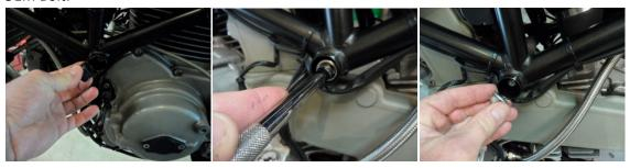
3. Slide the right hand slider (99-FS-750-8209-R) and spacer (428-9103) over the supplied engine stud as shown below and install engine stud through frame.
