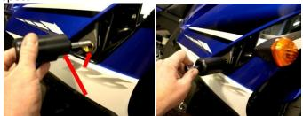
Remove left side panel. Remove left engine stud. Use 99-HB-SH10125070 Socket Cap 10 X 1.25 X 70 (Goes Though the Offset into the Frame) Main Engine Stud. Make sure your offset is at the correct angle so the puck will clear the body. Torque down to OEM torque specs.
