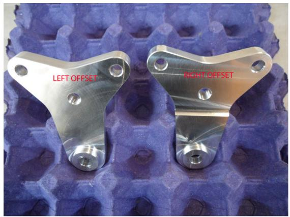
The photo above shows the back side of the offset (the side that will be facing the frame) you can see the right side offset has a radius step. This is so the offset will clear VIN tag on the right side of the frame.
