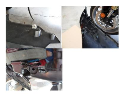
2. Attach the threaded frame cup spacers (99-SP-750-5410 x 2) to both left (99-OF-750-5450-L) and right (99-OF-750-5450-R) offsets using one drop of blue thread locker on the end of the 8mm (99-BH-0812520) socket cap button head bolts. Tip: Do not attach frame slider pucks.
