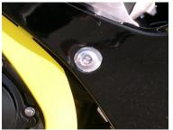
2. Attach the threaded frame cup spacers (99-SP-750-5410-L&R) to both left (99-OF-750-5410-L) and right (99-OF-750-5410-R) offsets using one drop of blue thread locker on the end of the 8mm (99-HB-0812520) socket cap button head bolts. Tip: Do not attach frame slider pucks.
