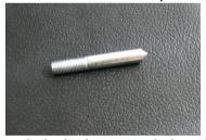
With the body removed, thread in by hand your spot tool. Make sure you have the spot tool screwed in enough to clear the body on the inside.
