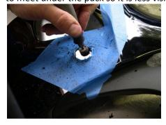
10. Mount right & left side puck with (99-HB-SH10125090) Socket Cap 10 X 1.25 X 90 Main Engine Stud and torque down to OEM specs.
