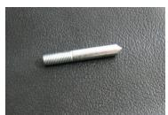
With the body removed, thread in by hand your spot tool. Make sure you have the spot tool screwed in enough to clear the body.
