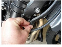
3. Install the right side offset using the 10x1.25x90mm bolt; lightly tighten up the bolt. Mount the right side body panel and position the offset so the slider puck will clear the bodywork. Mount the right side slider puck onto the offset using the 10x1.50x45 bolt to ensure correct location. Remove the slider puck and body work and torque down the offset bolt to the OEM engine bolt torque specifications.
